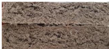
Figure 1. Cross-section of 3D cellulose pads.
