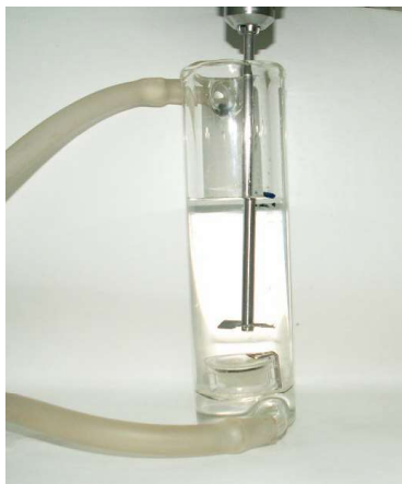
Figure 1. Paddle apparatus for testing in vitro the release rate of lidocaine hydrochloride from the polymer biocomposite hydrogels.
