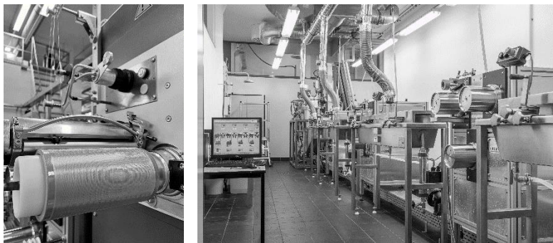
Figure 1: (left) Chitosan multifilament yarns spun with ionic liquids as a solvent; (right) Wet-spinning plant at the ITM
