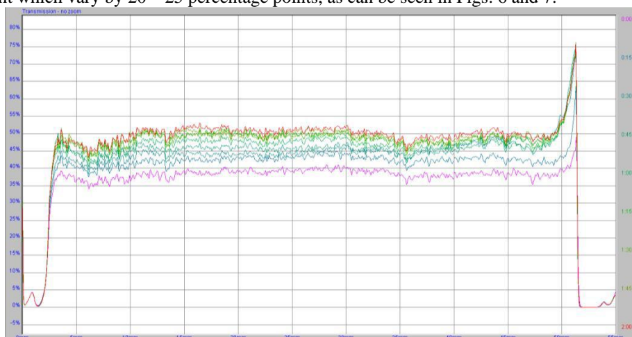
Figure 6. Transmission of light for titanium dioxide dispersion as a function of time and height of cuvette at pH 6. (start of measurements 0 min – pink; 15 min – dark green; 30 min – bottle green; 1 h and 1.30 min – different shades of green; 1.45 min – light green and 2 h – red, end of measurements). The X-axis reflects the height of cuvette, from 0 mm (bottom of cuvette) to 55 mm (top of cuvette).
