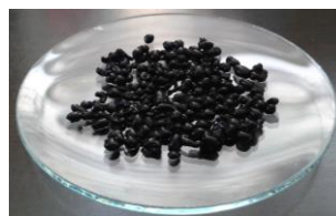
Figure 3. Activated carbon immobilised on chitosan
