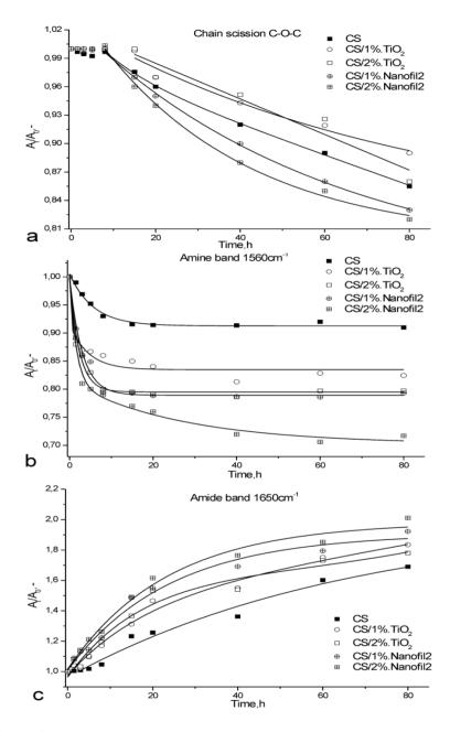
**Figure 2.** Relative changes of absorbance  $A_t/A_0$  of selected bands from FTIR spectra of chitosan and its composites with 1 and 2% content of TiO<sub>2</sub> and Nanofil2: (a) C-O-C (1080cm<sup>-1</sup>), (b) NH<sub>2</sub>(1577cm<sup>-1</sup>), (c) C=O (1655cm<sup>-1</sup>).
