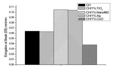
**Figure 3.** Elongation at break (EB) of chitosan nanocomposites before thermal treatment.
