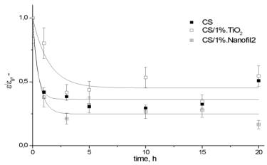
**Figure 4.** Effect of thermal treatment on relative elongation at break (EB) of the nanocomposites
