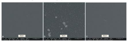
**Figure 1.** SEM photos of (a) chitosan, (b)  $chitosan/1\%TiO_2$  and (c) chitosan/1%Nanofil2 nanocomposites.
