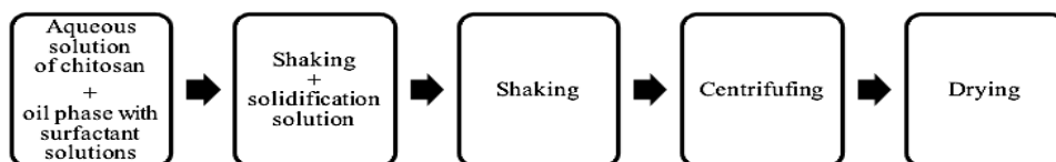
Scheme 3. The reverse micellar method for chitosan nanoparticle synthesis.
